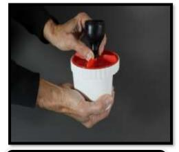
4. Thread the red flushing disk tightly onto the filter pack (if not already assembled).
