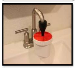
5. Press the flushing bulb onto a water faucet and run water for 4 to 5 minutes at low pressure.
