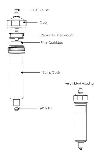
Rated Capacity: 1500 gallons or 12 months Maximum Working Pressure: 862 Kpa (125 psig) Maximum Working Temperature: 38° C (100° F) Minimum Operating Pressure: 69 Kpa (10 psig) Minimum Operating Temperature: 5° C (41° F)
